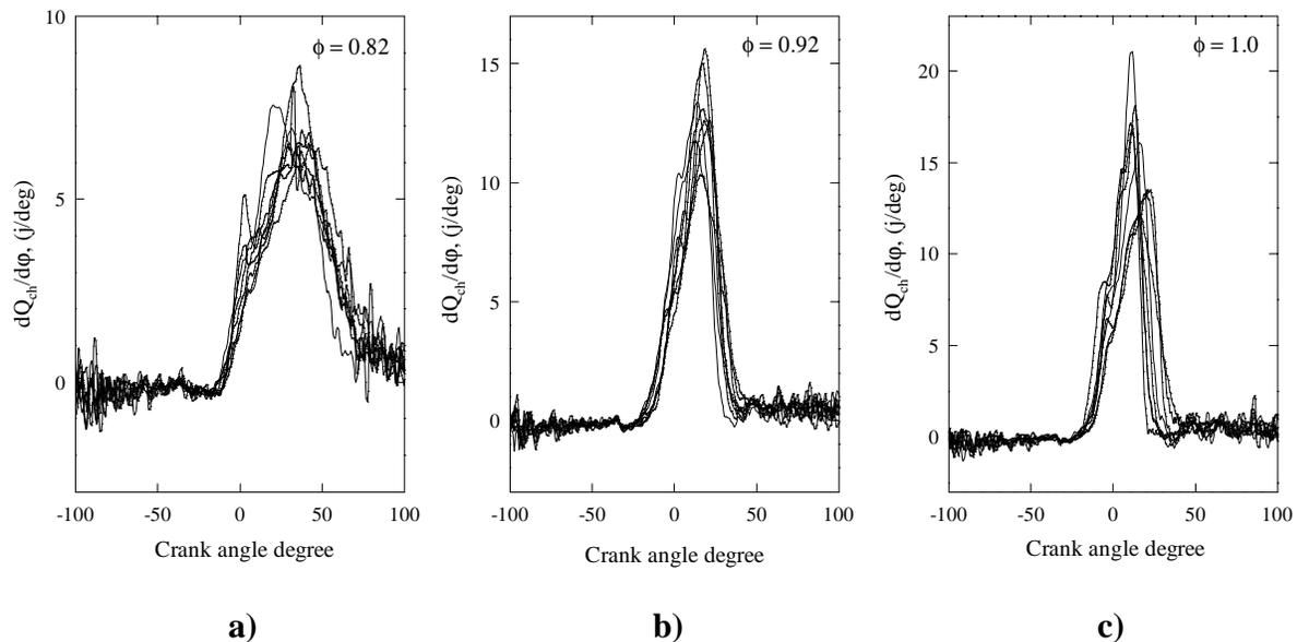
Figure 4- Gross heat release rate per crank angle degree: a)  $\phi = 0.82$ , b)  $\phi = 0.92$ , c)  $\phi = 1.0$
