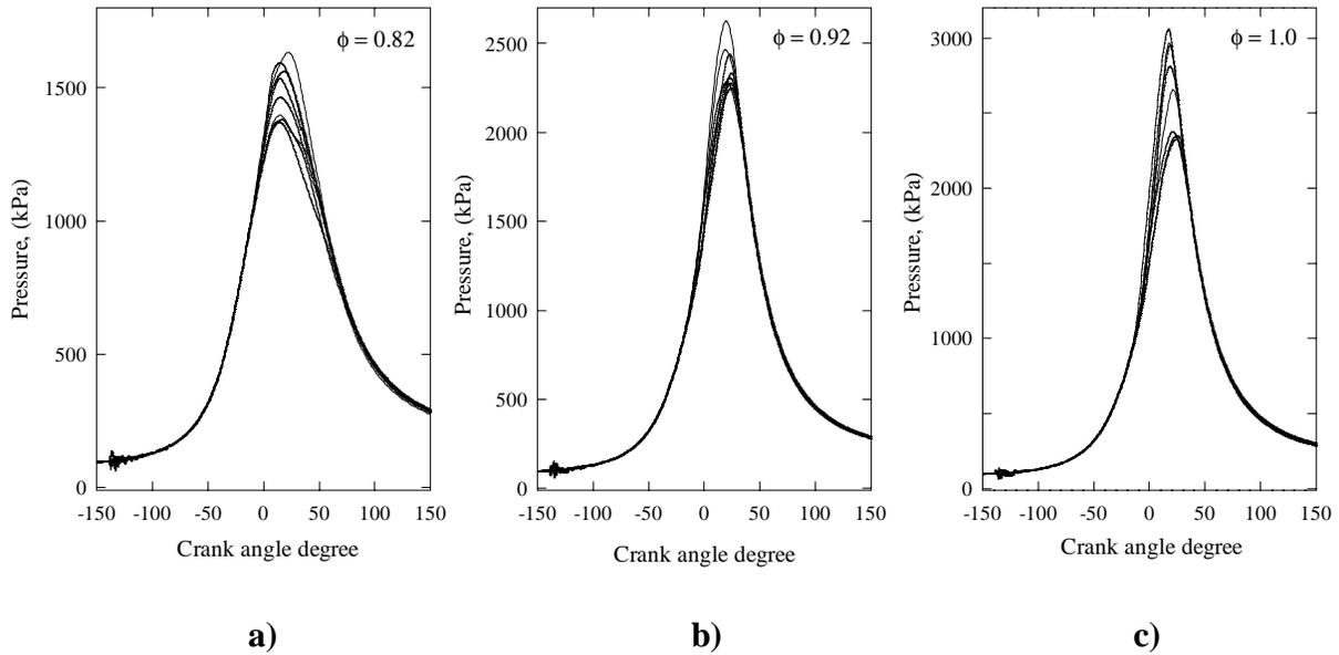
Figure 2- Cylinder pressure per crank angle degree: a)  $\phi = 0.82$ , b)  $\phi = 0.92$ , c)  $\phi = 1.0$
